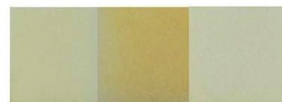
No stabilizer Amine stabilizer Amine-free stabilizer
