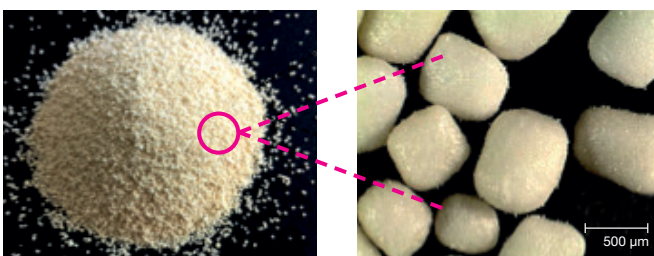
FIGURE 4: NATUPHOS® E GRANULATES ARE VIRTUALLY DUST-FREE AND HAVE A NARROW PARTICLE SIZE DISTRIBUTION
